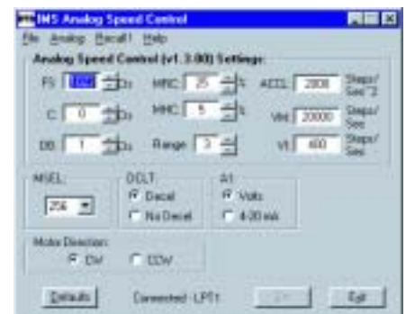
The IMS Speed Control Interface GUI simplifies MDrive configuring with a single screen interface.
